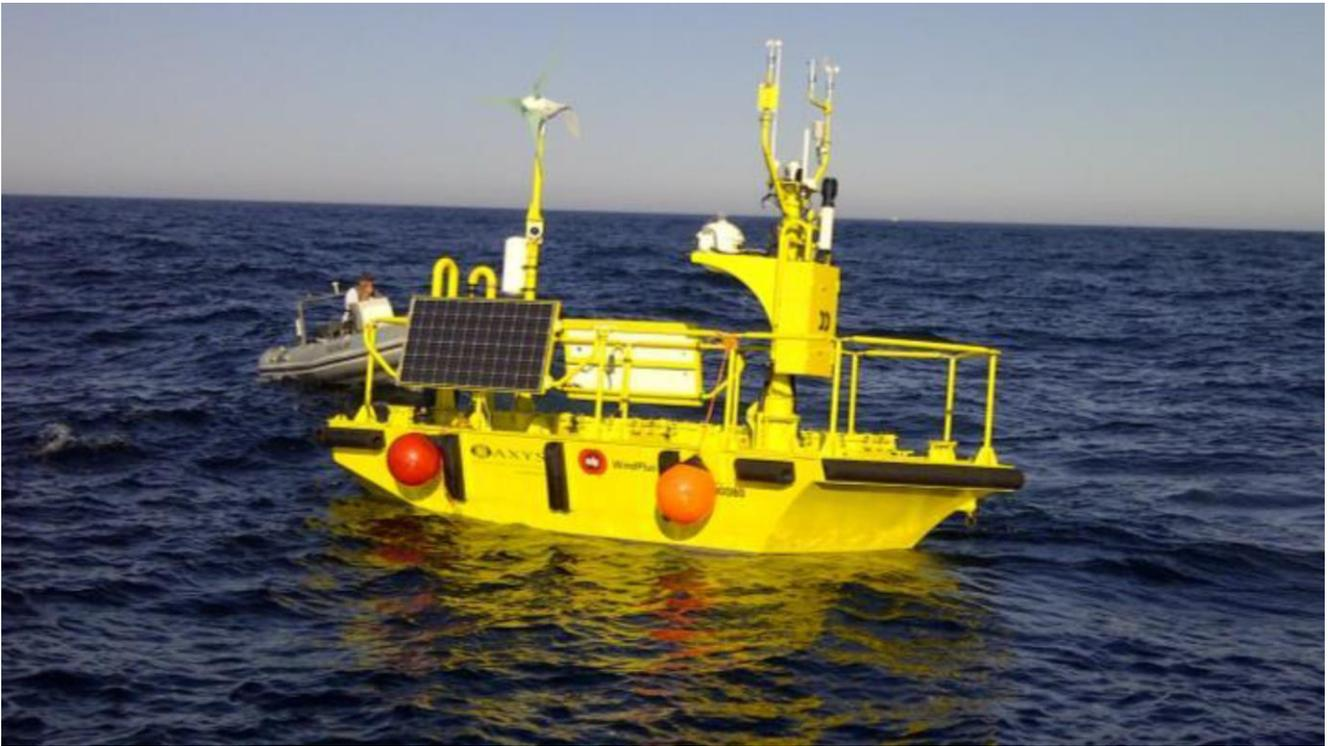
***AXYS Floating LiDAR Buoy***
