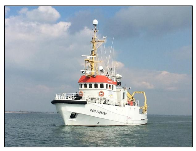
The 'EGS Pioneer' is a 24.4m dedicated survey vessel owned by EGS and equipped to undertake coastal survey work. The vessel operates under the UK Workboat Code (Cat2).
